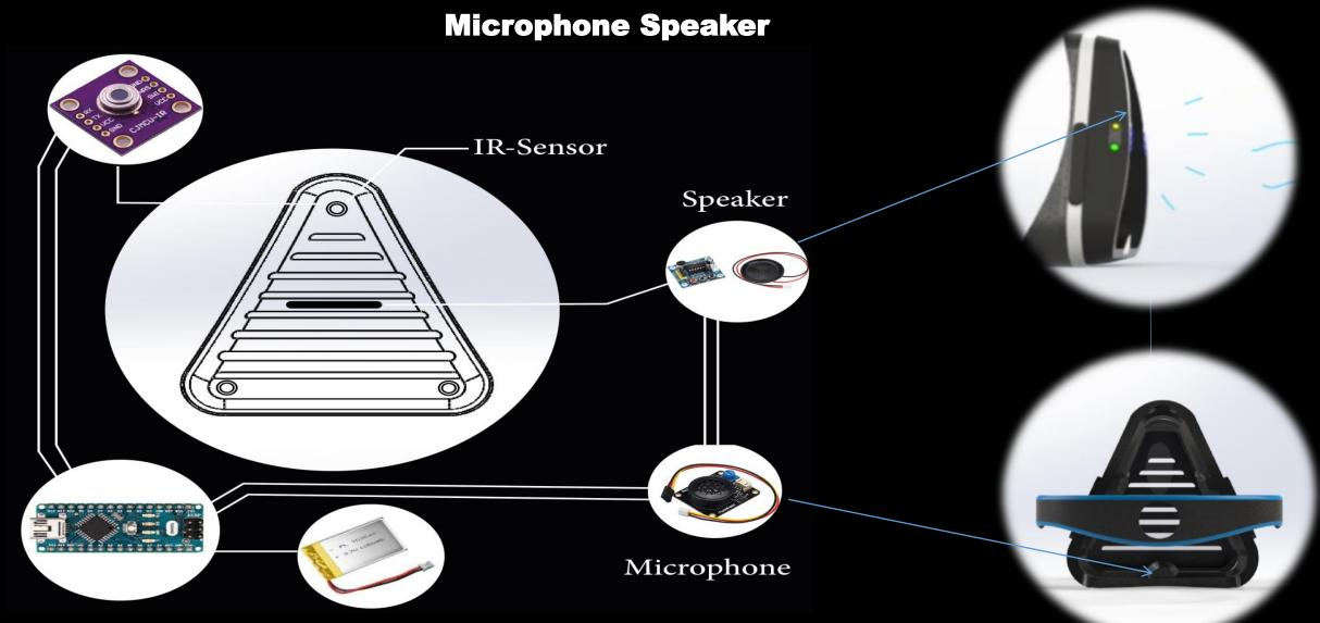
This inbuilt system amplifies the volume of voice to be easily heard while communicate over distances, making the person heard clearly. (up to about 10 meters range)
